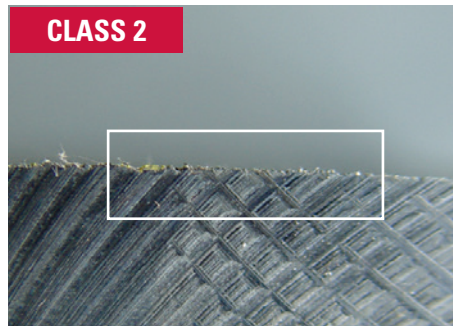
Feather burrs are readily visible without magnification and are characterized by extremely thin roots. They can be removed with a tip of a pencil.
